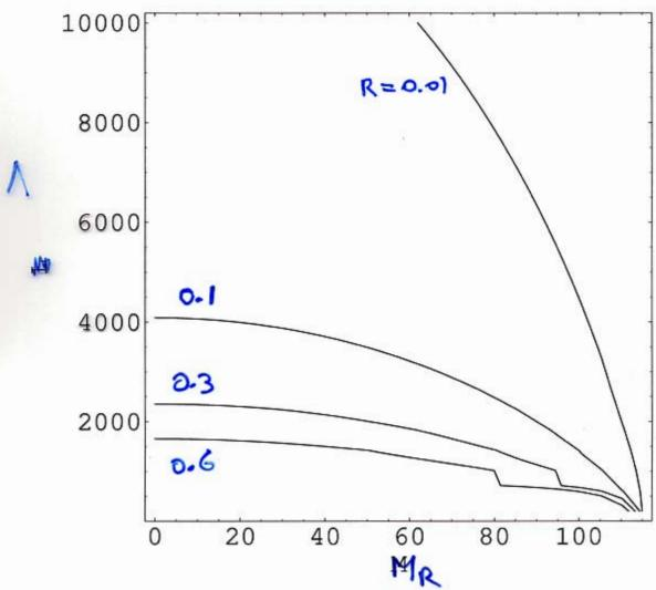
Have seen that, if kinematically allowed, the higgs boson can have significant branching fractions into right-handed neutrinos. Can be the dominant decay channel.
