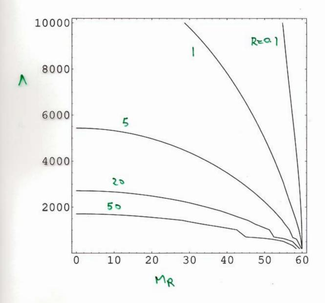
$R = \Gamma[h \to \nu_R \nu_R]/\Gamma[h \to b \bar{b}] \ , \ m_h = \text{150 GeV}$
