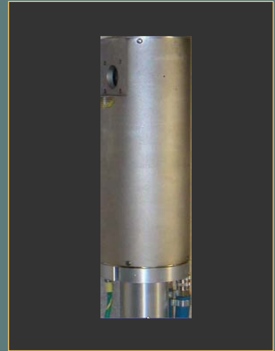
Comet 1 kW Tube 12.5 mA at 80 kVp
