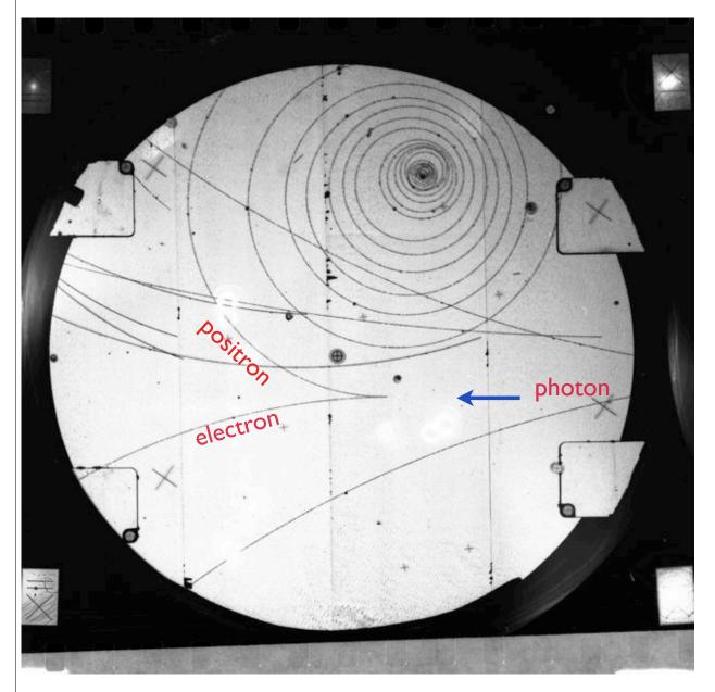
Photon incoming converts to electron (-) and anti electron (+) (called a positron)
