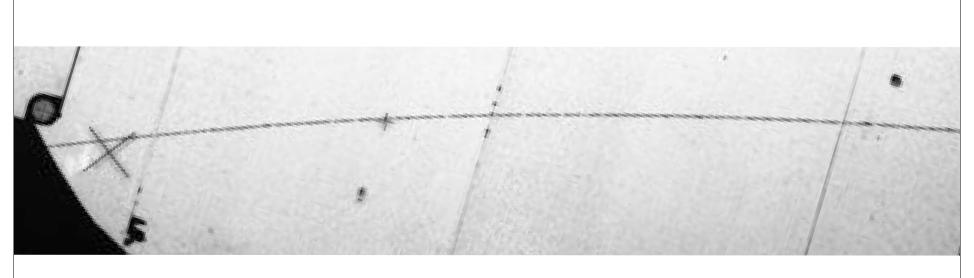
Can almost see individual bubbles along track Note no bubbles in the bulk of the liquid Some bubbling starting at cracks on the bottom
