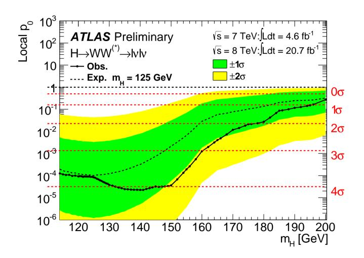
small additional excess for  $M_H \gtrsim 135$  GeV (low mass resolution)
