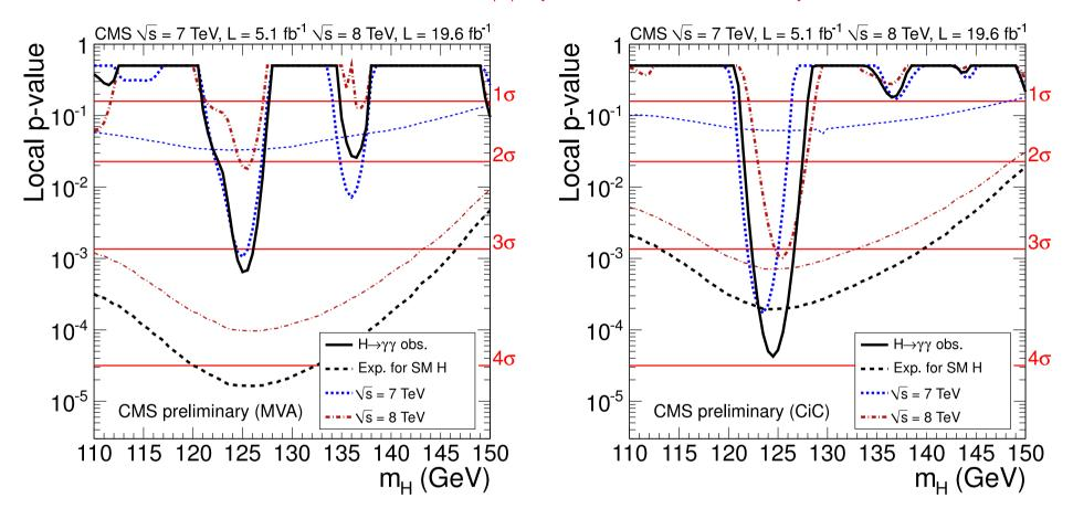
Either: an additional  $\sim 2\sigma$  excess around  $M_H \sim 136$  GeV (MVA analysis, l.h.s.), or confirmation of the enhanced  $\gamma\gamma$  rate of the 125 GeV Higgs (cutbased analysis, r.h.s.; still:  $\sim 1\sigma$  excess around  $M_H \sim 136$  GeV)
