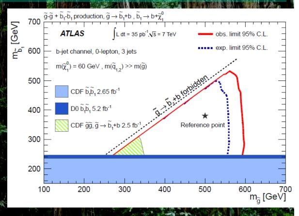
Quasi-model-independent limits in gluino-sbottom plane
