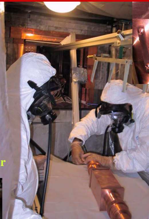
installing DAMA/LIBRA detectors
