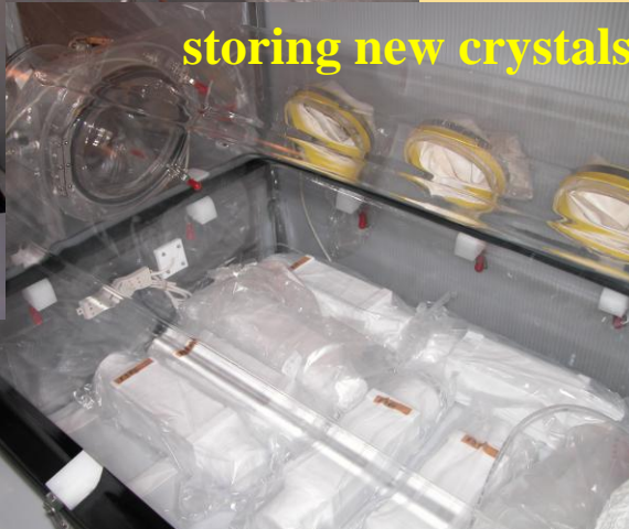
Cu etching with super- and ultra- pure HCl solutions, dried and sealed in HP N 2
