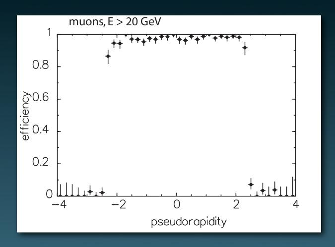
efficiency about 97% out to |η| = 3 (depends totally on track efficiency)
